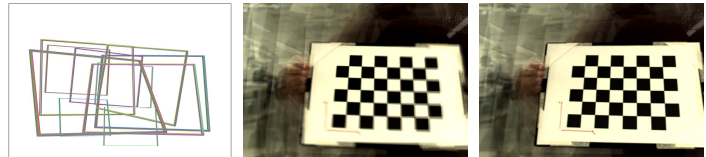
(a) All imaged chessboard poses (b) Merged after linear solution (c) Merged after nonlinear solution
