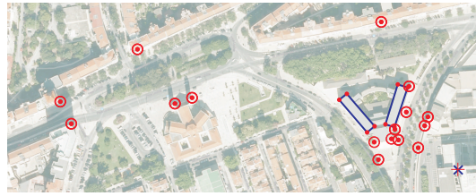
(b) Aerial view (Google maps) and horizontal (blue) and vertical lines (red dots) used for calibration.
