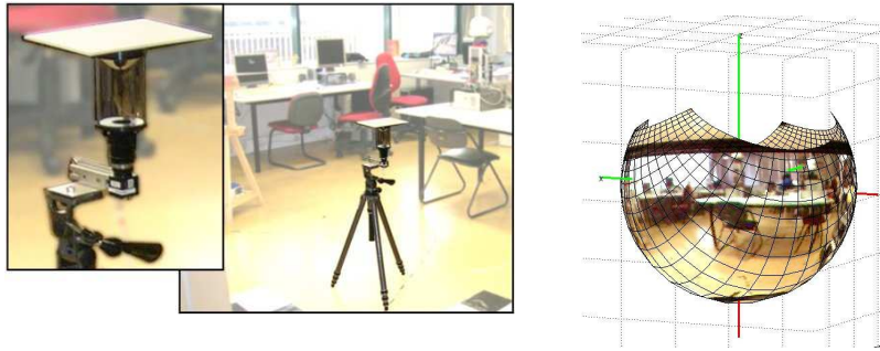
Fig. 3. Left: The camera used to sample omnidirectional images (image mirrored). Right: A calibrated omnidirectional image mapped to a sphere.
