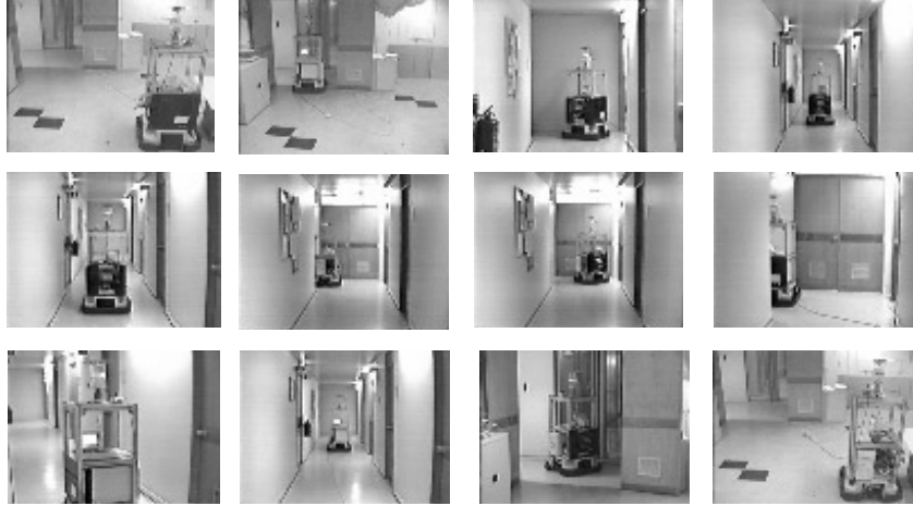
Figure 16: Experiment combining visual path following for door traversal and topological navigation for corridor following.
